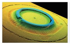
Inspection Content : Defects such as pinholes, partial welding, broken welding, fmissed welding, warped nails, no nails, etc. Detection Accuracy : 0.2mm Visual Detection Range : ≤ 9mm Overkill Rate : < 1.0% Omission Ratio: 0 Equipment Beats : ≤ 6.3PPM Visual Beats : ≤ 1.5s/PCS
