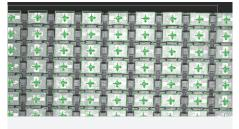
Frame Width : ≥ 135mm Product Size : ≤ 320mm×135mm Chip Size : Minimum 3mm×3mm, Maximum 65mm×65mm Image Acquisition Time : ≤ 3s Image Processing Time : ≤ 30ms / Single Chip Visual Positioning Accuracy : ≤ ±0.02mm
